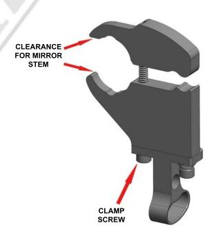
STEP 2 - Loosen the CLAMP SCREW so there is enough clearance between the TOP and MID SECTIONS to slide over the mirror stem.
